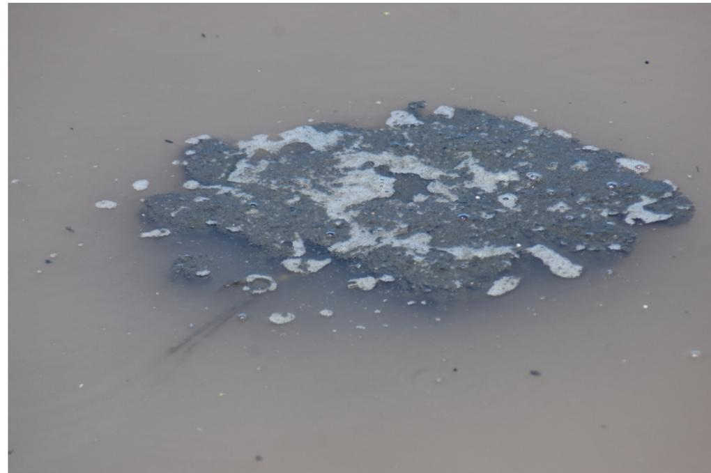
Sludge that is dark and has been starved of oxygen is more likely to produce hydrogen sulfide, which has a distinct “rotten egg” odour. This material will be targeted in the removal process.
