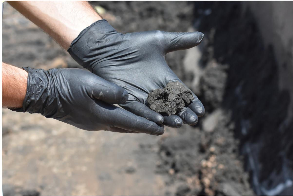
Up to 8,400 tonnes of sludge is being removed from the primary lagoon. This is what it looks like after it is dewatered.
