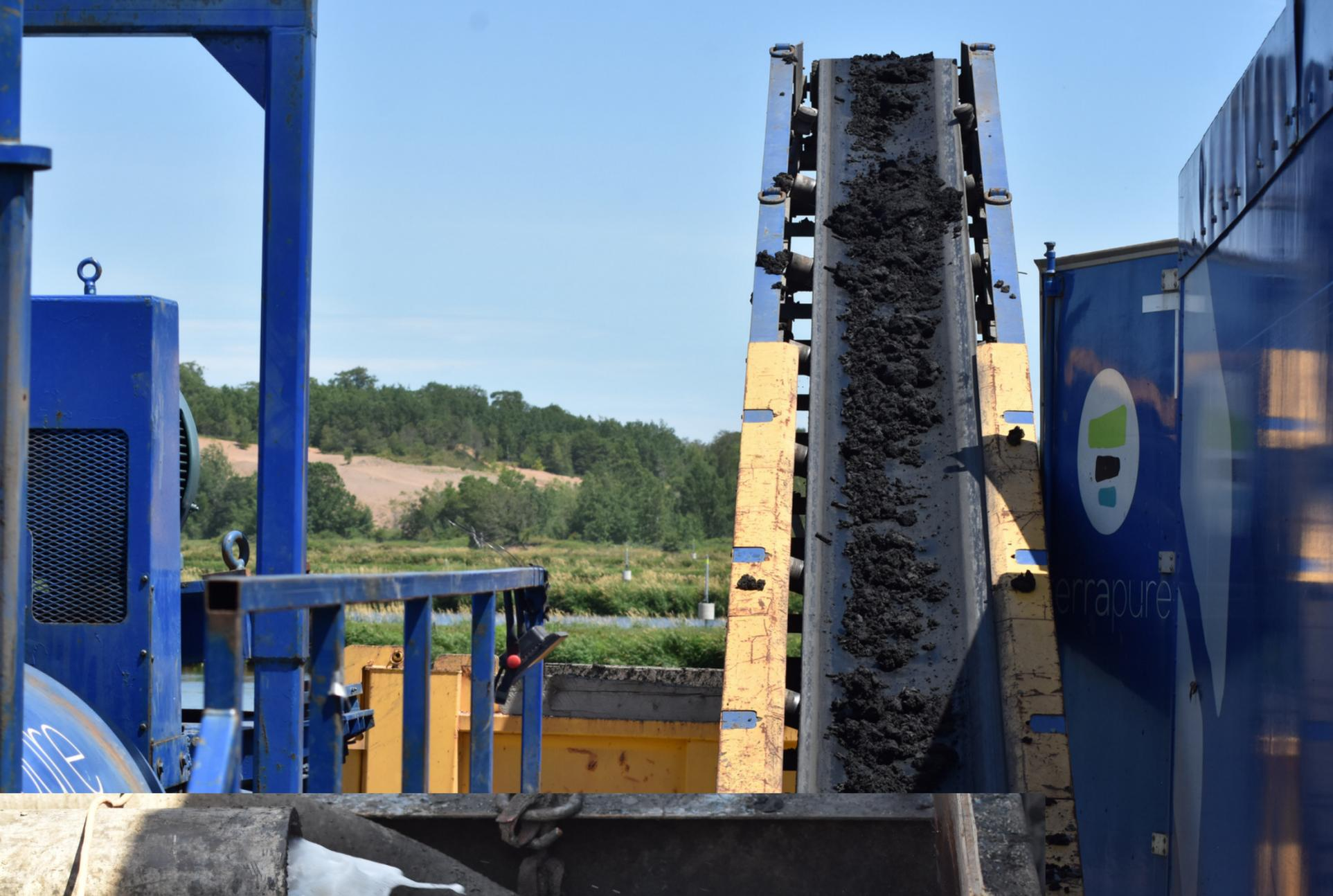
The sludge extracted from the primary sewage lagoon is cycled through a spinning centrifuge for dewatering.
